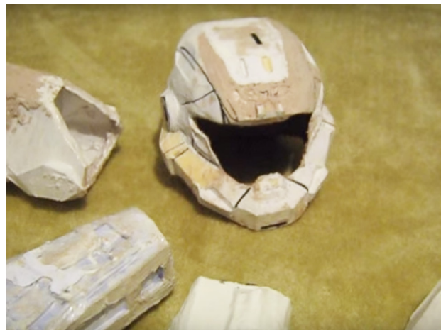
This fibreglassed pepakura pattern needed a lot of finishing work before I could paint it.
