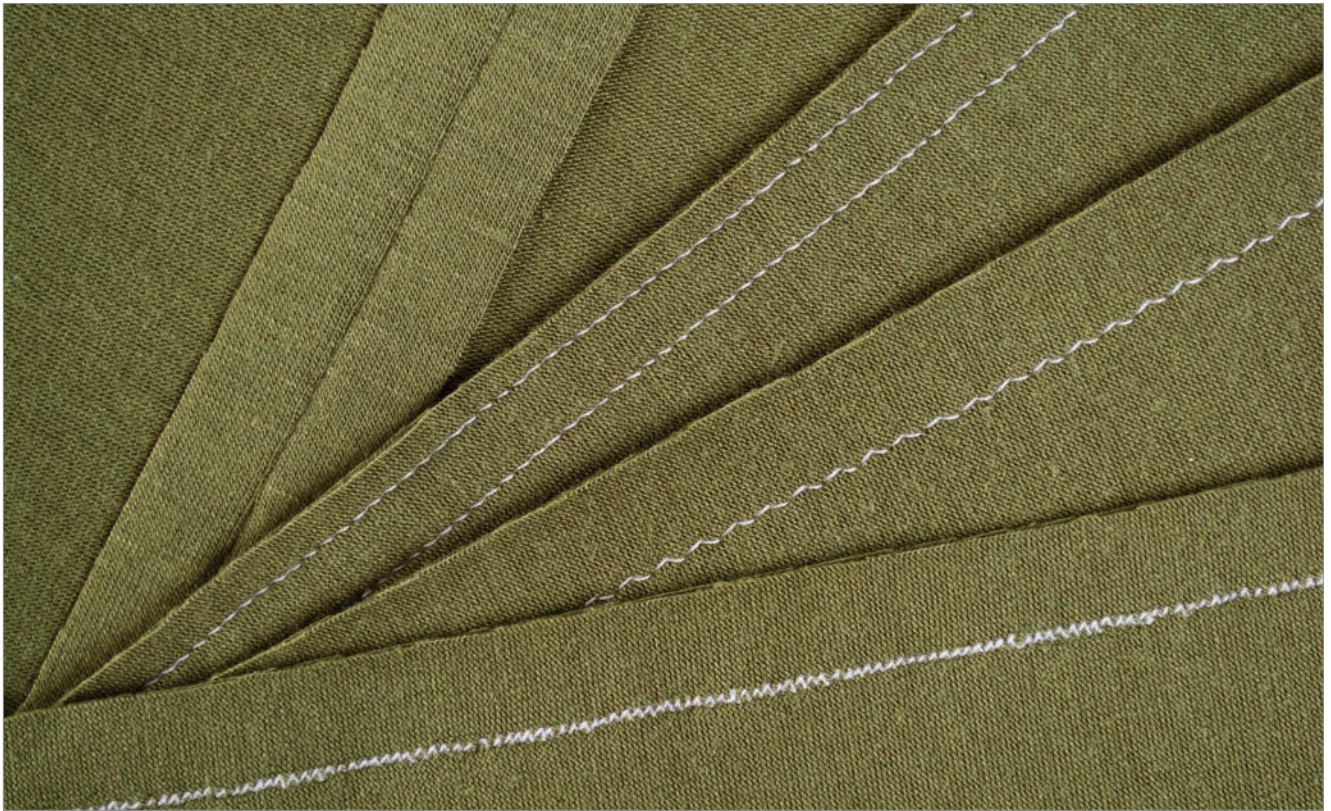
Samples of four sewing machine seam finishes (from top): Straight stitch with seam pressed open, double-stitched, zigzag stitch, and programmed knit stitch.
