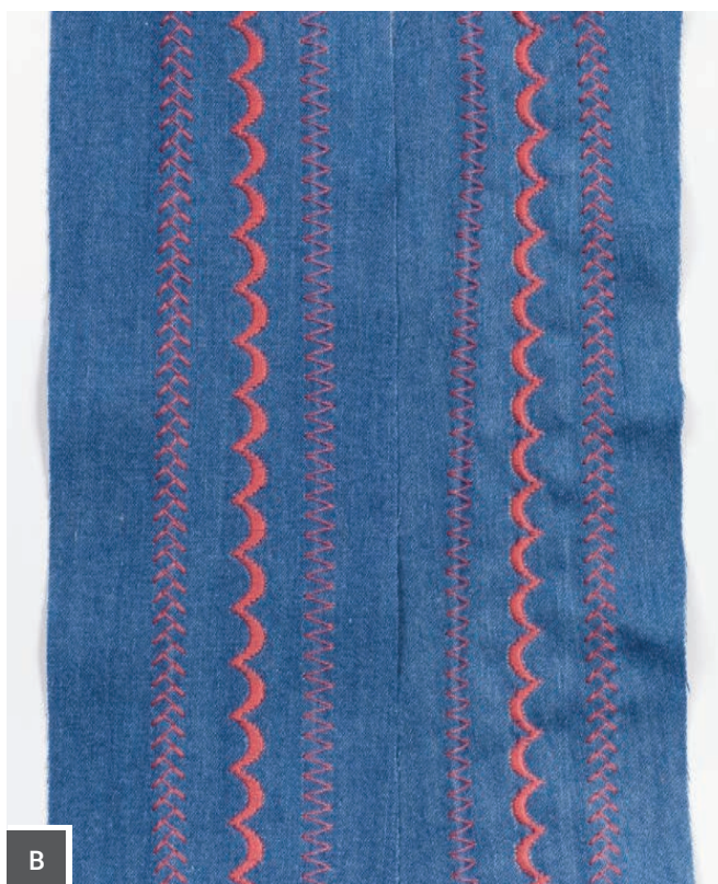
Stitches made on fabric with (left) and without fusible tricot interfacing.
