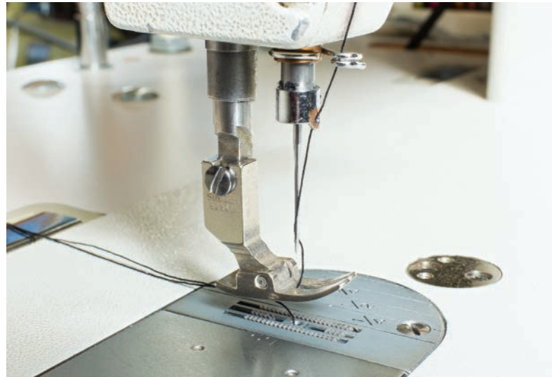
High shank feet are typically used on industrial machines and older model (pre-1980s) domestic machines. Super high shank feet are found on some vintage Kenmores and they look like slant shanks on steroids!
