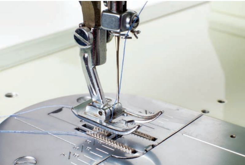
Slant shank feet are found only on Singer machines from the 1960s and '70s.
