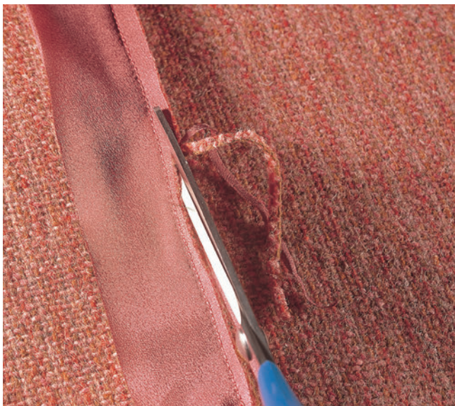
3 Trim seam allowance of heavy fabric to \frac{1}{8} " (3 mm) to reduce bulk. Lightweight fabric does not need to be trimmed.
