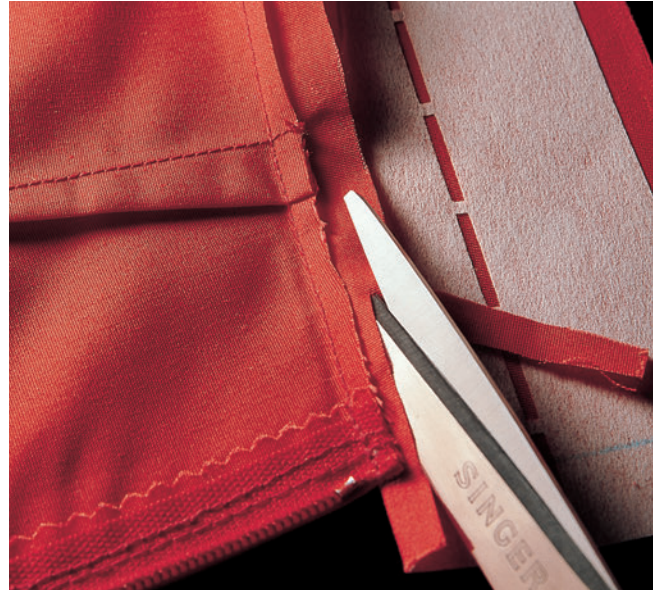
6 Grade the seam allowances to \frac{1}{4} " (6 mm) on the waistband and \frac{1}{8} " (3 mm) on the garment to eliminate bulk.
