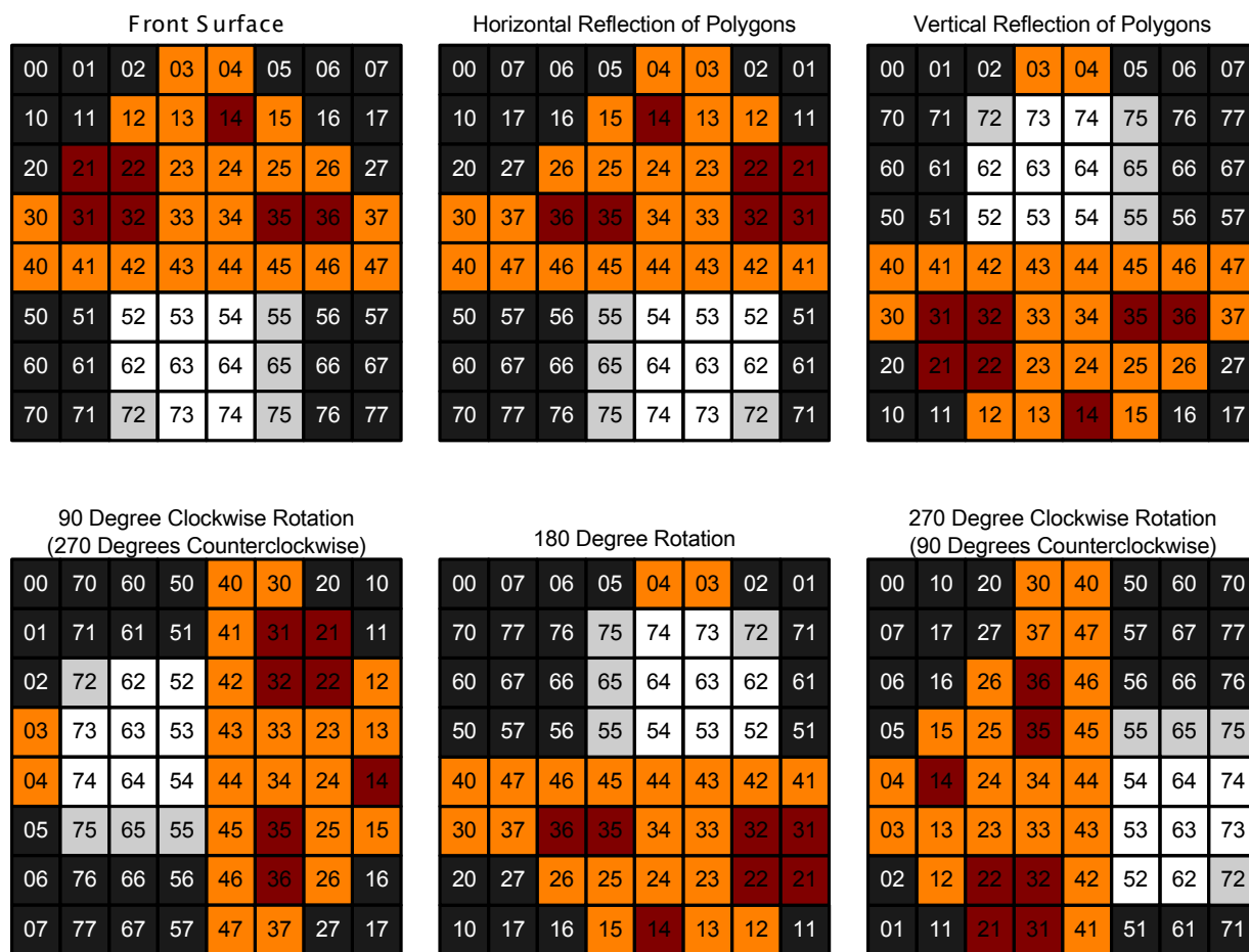
Figure 6-39 : Displaying Front and Back Surfaces of an LCD
